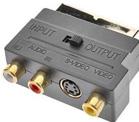
The :SCART to RCA plug converts your SCART output to the more common RCA plug. IMPORTANT: If it is switchable, make sure that the switch is set to OUTPUT (see picture)!
