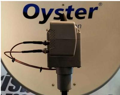
Above is a picture of an LNB in the parking position. Notice the 2 coax cables pointing to the 9 o'clock position. The LNB should move into this position when the dish is retracting AND move out of that position when the dish is opening. This is critical!
