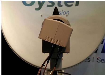
Above is a picture of an LNB in the 7 o'clock position, which is the correct position for the East Coast of Australia.
